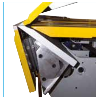
Excellent clearance of the bending apron due to wide inclination angle
