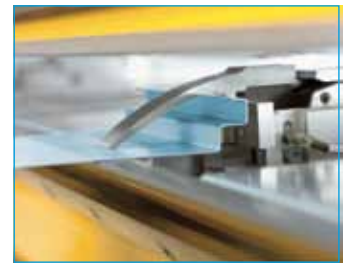
Individual customised gripper fingers for changing – Stop fingers for very low supporting surfaces of the plate of .196 inch - .945 inch
