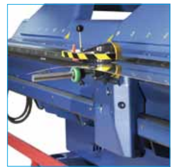
Powerful automatic cutter with quick lever thickness adjustment
