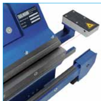
Laser monitoring of the clamping range
