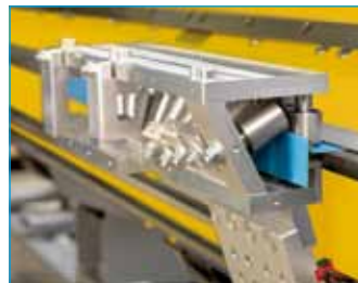
Customised roll forming tool for special profiles
