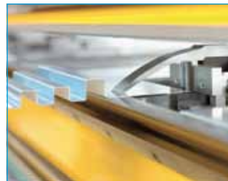
Individual customised gripper fingers for changing – Stop fingers for very low supporting surfaces of the plate of 5 - 24 mm
