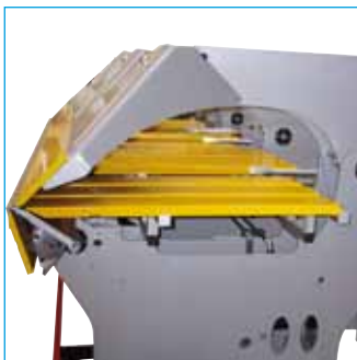
On coil gauge aligned inlaid depth of 1250 mm
