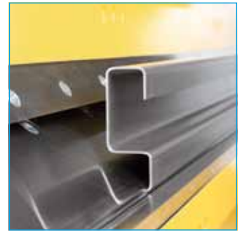
Precise bending even with 3 mm sheet steel (400 N/mm 2 )
