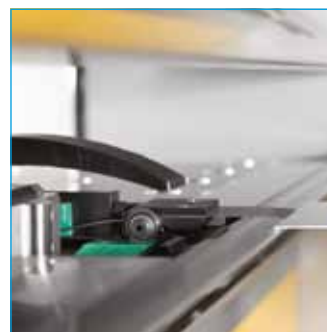
Back gauge finger with minimum working dimension of 5 mm
