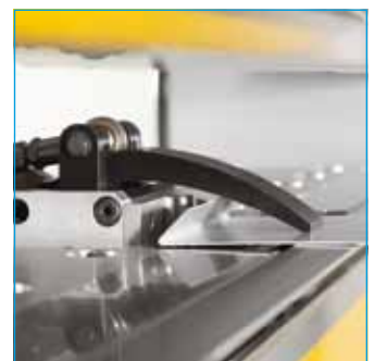
40 mm gripper-span to hold even bended parts
